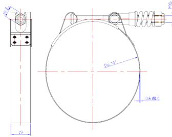
Recommended Installation Torques: 12Nm / 9Nm
