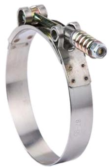
**GABBTECH** Spring loaded T-bolt clamp is designed to compensate for pressure fluctuations in all types of hoses. When temperature, pressure, or tension strength changes cause the hose line to expand or contract, the spring-loaded bolt and barrel hose clamp can adjust accordingly to provide constant band tension.
